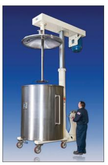
Vacuum-design high-speed disperser with air/oil hydraulic lift for easy access into the 600-gal mixing vessel.
