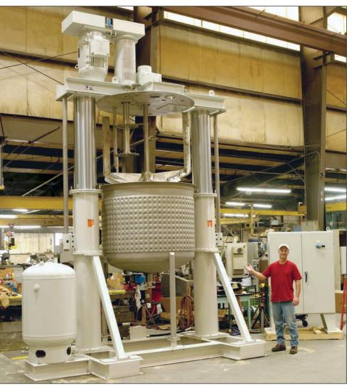
500-gal multi-shaft mixing system with independently controlled high-speed disperser and anchor agitator.
