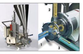
Inline rotor/stator mixer designed for sub-surface induction of fine and difficult-to-wet powders. The liquid stream (1) enters the mixer and immediately encounters powders being drawn into the mix chamber by a powerful vacuum generated by the ported rotor (2). The resulting dispersion (3) is expelled centrifugally through the stator openings at high velocity.
